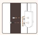
**Step 1:** Pull tension device down to where there is very little slack. Mark the area where the bracket sits.
