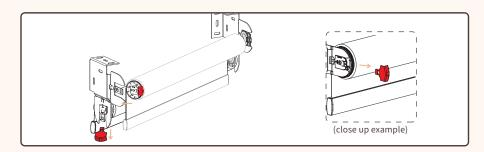
When installing cordless version, insert bearing side following with the side that has the red clip (spring lock), if needed reference page 1 "installing shade" for guidance. It is important to note not to remove the lock on the tension side before installing. When installed the red clip will pop off.
