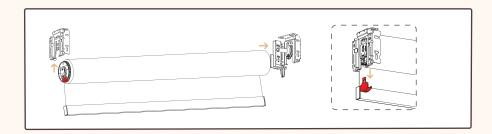
When installing cordless version, reference the same steps on page 1. The side with the spring lock (red clip) is to be installed after the bearing side. The lock will pop off once installed. Do not remove the lock before the shade has been installed.
