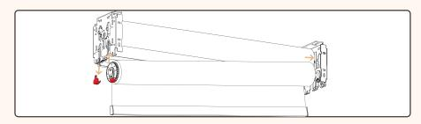
When installing cordless version, refrence the same steps on page 1&2. The side with the spring lock (red clip) should be installed after bearing side. The lock will pop off once installed. Do not remove the lock before the shade has been installed.
