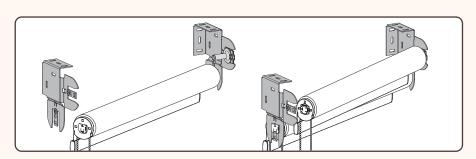
Begin with installing bottom roll first, insert bearing pin side and follow with the control side. Once snapped in to place, repeat with the top roll.
