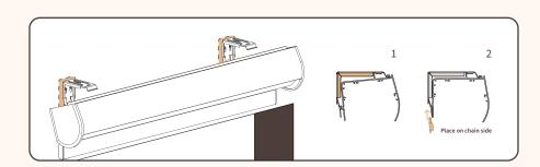
Begin with sliding shade in back end lowered with back end lowered enough for lip of bracket to make contact with lip on top of cassette. Once contact is made beg in to lift back end up until you hear a click.
