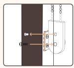
**Step 1:** Pull tension device down to where there is very little slack. Mark the area where the bracket sits.
