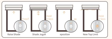
**Setting Top Limit:** To adjust the top limit, raise the shade to the preset top position. Press and hold the up and down button simultaneously until the shade jogs. Reposition the shade to the desired top limit. Press and hold the My button for 2 secs to confirm the new bottom position. The shade will then jog, confirming position.
