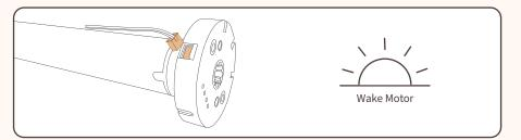
Activating Motor: When shipping the shade will be placed in a sleep mode. Wake up shade by connecting the motor to the charger. The shade will briefly jog up/down. Motor will now operate with programed transmitter.
