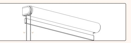
**Lower/Raise:** Continuous loop controls have a chain that loops back into the clutch. To **lower** your shade, pull down on the back of the chain. To **raise** your shade, pull down on front of the chain to lower.
