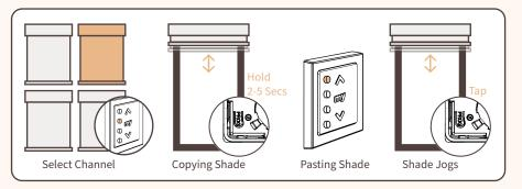
Adding Shades To Channels: To add a shade to a channel. Select the channel that your shade is currently programmed to. Press the program button on the back of the remote for 2-5 seconds. The shade will jog. Program within 2 mins or shade will reset to factory settings.
