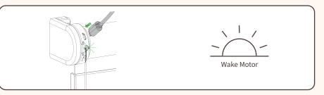
**Activating Motor:** When shipping the shade will be placed in a sleep mode. Wake up shade by connecting the charger to the shade motor.
