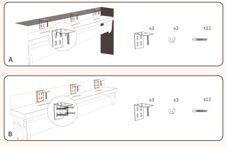
**A. Inside Mount:** Measure from the left end of board to the middle of left slot. This is the distance you will want to center and install your bracket from left side of window casement. Repeat process for middle and right brackets. For mounting shade flush to window casement, do not install bracket within a minimum of .75" of outer end of window casement.
