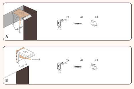
**A. Inside Mount:** Install brackets minimum of 2" from the side of the window frame.
