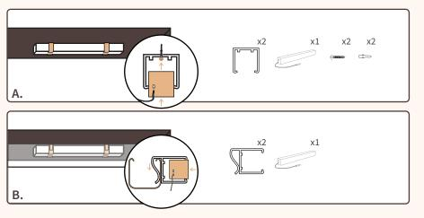
**A. Wall/Ceiling Mount**: Using the bracket with the screw slot, install battery behind shade and directly in to window casement. Make sure to use anchors if driving screws directly in to dry wall.
