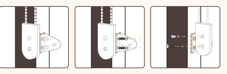
**Step 1:** Pull tension device down to where there is very little slack. Mark the area where the bracket sits.
