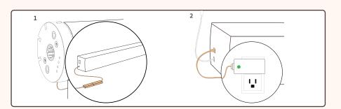
Power the motor by connecting the two exsiting cables from the motor and the battery together. To charge the battery, plug in the provided charger to a nearby outlit and plug charging cord in to charging port of battery. (Disconnect battery from motor if provided charger does not reach.)
