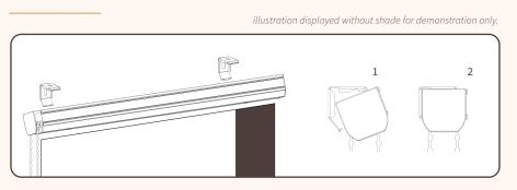
Begin with sliding shade in back end lowered with back end lowered enough for lip of bracket to make contact with lip on top of cassette. Once contact is made beg in to lift back end up until you hear a click.
