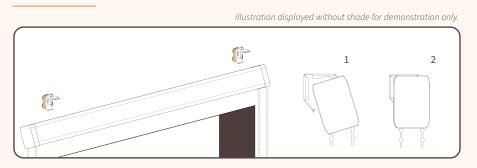
Slide the shade in to the brackets with back end of headrail at an angle. Allow the front lip of bracket to slide under the front lip of the top of the headrail. Then press the back of headrail up firmly in to the bracket until you hear a click.
