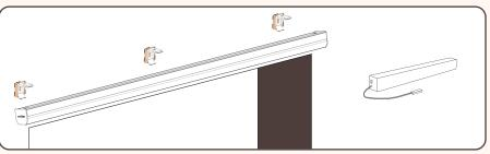
**Slim Fit Motorized headrail** is installed the same way as **Slim Fit**. When installing motorized version you must also install **Battery Pack**.
