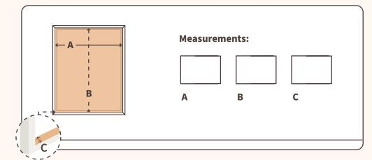
**Step A** - Measure the top width inside the window opening. If tiles or other materials cover part of the inside of the opening, consider measuring the opening at its narrowest spot and record that measurement.
