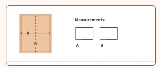
**Step A** - Measure the width of the window opening. For windows without trim add 2-4" per side, for windows with trim measure to outer edges of trim.
